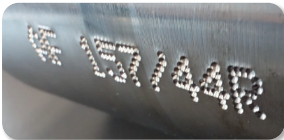
■ Deep marking on beams / tubes / chassis
